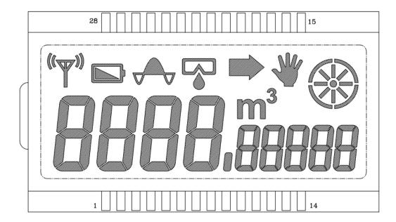
The total amount of water consumption appears permanently on the meter's display. In detail, the four large figures indicate number of cubic meter and the five small figures are decimals.
